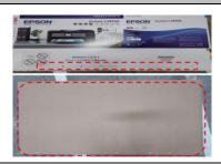
INHOUSE DETECTION: Glue Stain LOT SIZE: 300 PCS REJECT QUANTITY: 140 REJECTION RATE: 46.67% JO: 25010 REMARKS: Glue Stain occured on the bottom flap and on the back surface of the panel.
